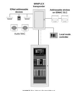
Figure 1: Typical 4100ES MINIPLEX System One-Line Drawing
